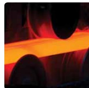
Above: Cast bar in copper rod plant, Sterlite.
